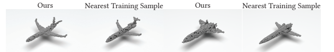
Fig. 27. Generated airplanes (left of each pair) and their nearest training samples under Chamfer Distance (right of each pair). The generated shapes are visually distinct from their closest training neighbors, indicating that the model produces novel geometry rather than memorizing training data.
