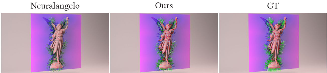
Figure 24. SDF Curvature (Lucy) . Mesh colored by mean curvature, green lines show gradient direction. Hermite-NGP achieves gradient MAE 0.0418 vs. NeuralAngelo’s 0.1213 ( 2.9\times lower).
